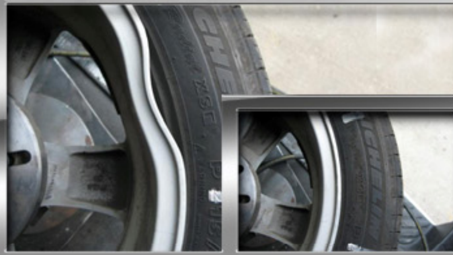
Gouged and Bent Wheels
